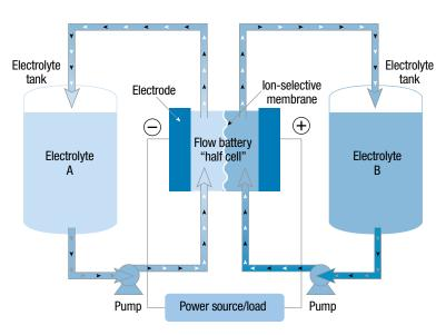
AvCarb PAN-based carbon and graphite felts are used as electrode backings in a variety of battery designs including vanadium redox flow batteries. AvCarb supports the needs of advanced battery makers with highly uniform carbon felts that ensure reliability and durability of the electrochemical system. The high conductivity, high purity, and chemical resistance of AvCarb battery felts make them ideal for the demanding design criteria of flow battery developers.
