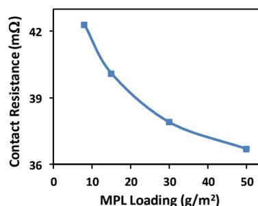
Figure 5. Influence of MPL loading on contact resistance as measured via TLM
