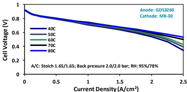
Figure 8. Single cell polarization curves at different operating temperatures
