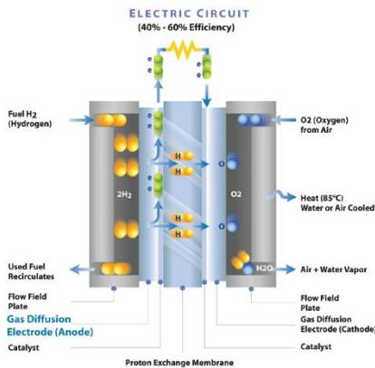
Figure 2. Schematic of fuel cell operation
