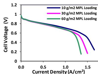
Figure 4. Influence of MPL loading on cell performance under wet operating conditions (> 70% RH)
