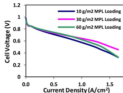
Figure 3. Influence of MPL loading on cell performance under dry operating conditions (< 30% RH)
